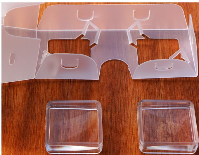
Maintaining the orientation, clip the right lens (left in the figure) in position, pushing the two 'goalposts' firmly over the corners so the lens is held tight. Repeat for the left lens, to give:
